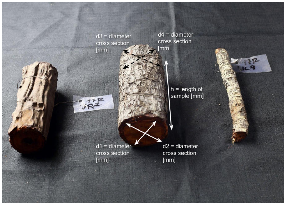
Figure 25: Samples taken from section: stilt root, trunk and crown of tract no. '17. Measurements for the volume determination explained on the trunk sample (Forstreuter, 2017).
